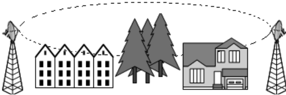
FIGURE 13-7: Path loss. The elliptical path between endpoints should be clear from obstruction.
